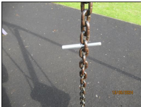
(Openings in chains exceed 8.6mm)
